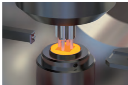
TPD Workstation with hot sample
